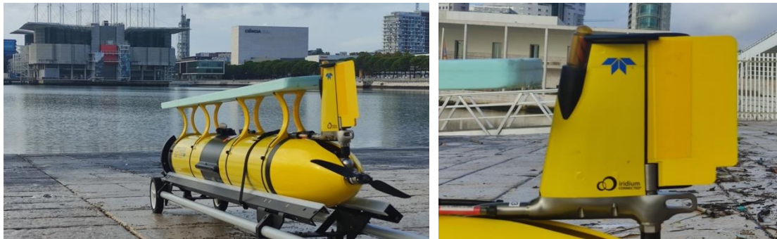
Figure 16: Glider equipped with contraction for added floatability (left) and detail of rudder extender (right).
