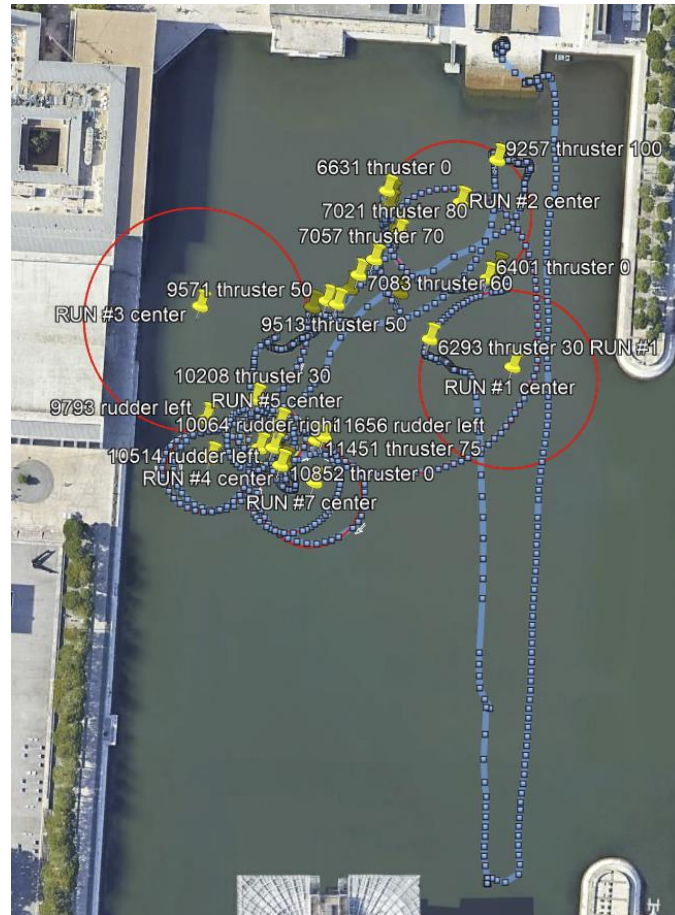
Figure 19: GPS data points during the trials. The range test (top-to-bottom segment and back) and several arc-circles (full circles overlaid in red) are clearly visible.
